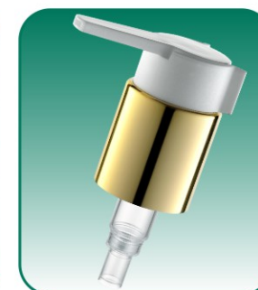
HB-502M Specification: \Phi 22/410 \Phi 24/410 Discharge Rate: 0.5 \pm 0.05\text{ml/T}
