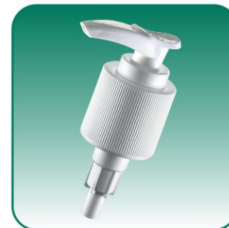
HB-217H Specification: \Phi 28/415 Discharge Rate: 1.8-2.2ml/T
