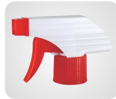
HB-710 Specification: Φ28/400 High:17mm Φ28/410 High:21mm Φ28/415 High:25mm
