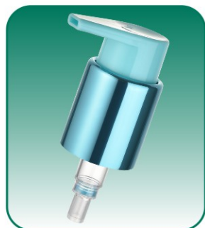
HB-511H Specification: \Phi 22/415 , \Phi 24/415 Discharge Rate: 0.5 \pm 0.05\text{ml/T}
