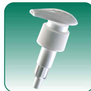
HB-215A Specification: \Phi 24/410 Discharge Rate: 1.8-2.2ml/T
