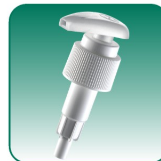
HB-222A Specification: \Phi 24/410 Discharge Rate: 1.8~2.2ml/T
